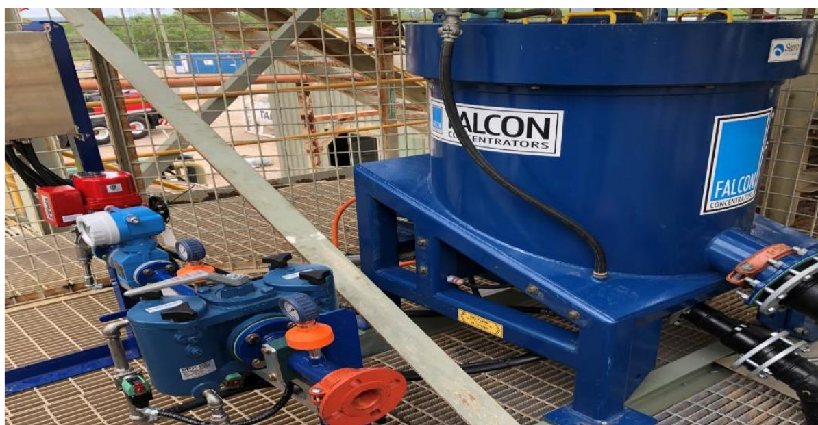
Figure 3: SB750 Falcon Gravity Concentrator (part of gravity gold recovery circuit)
