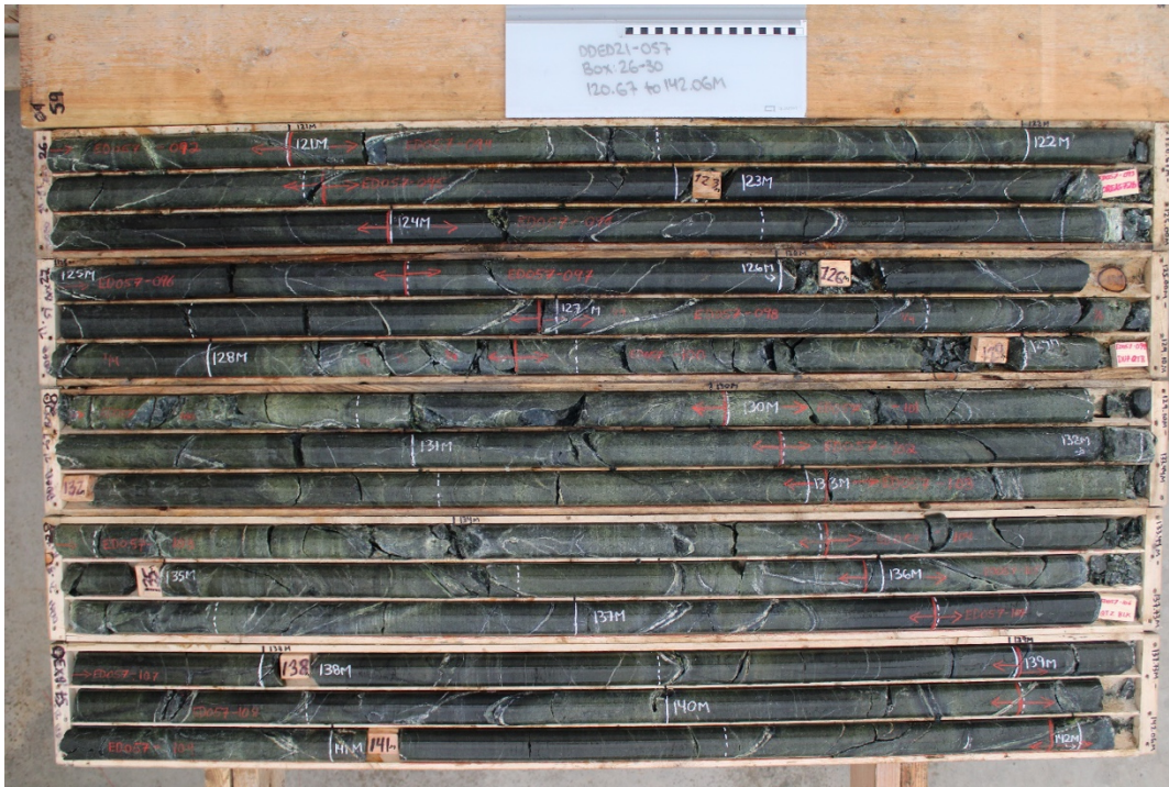
Figure 5: DDED21-057: Serpentinized peridotite, dunite host unit with trace disseminated sulphides
