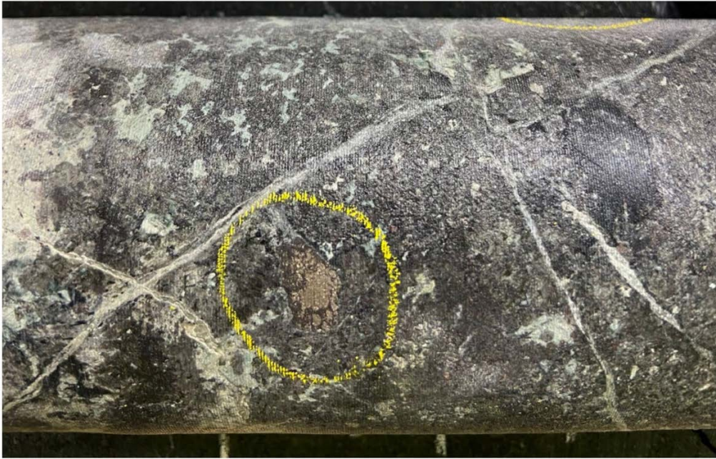
Figure 6: DDED22-085, Blebby heazlewoodite-millerite within pyroxenite at 151.34m
