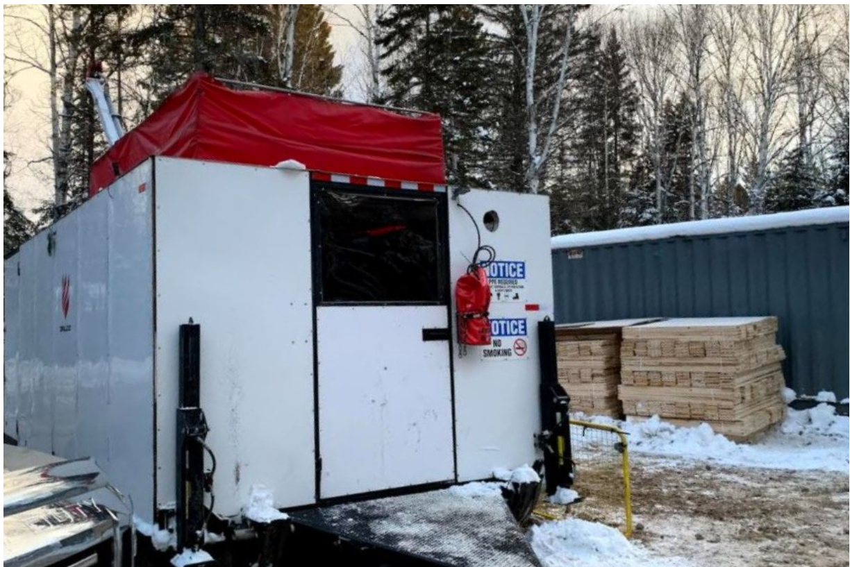
Figure 1: Winterised Diamond Drill Rig Located on Site at Edleston
