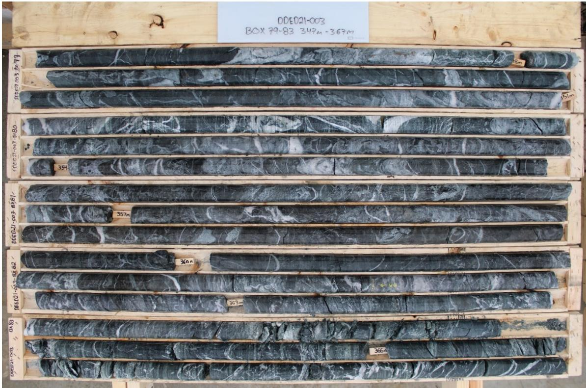
Figure 4b: DDED21-003 Boxes 79 - 83, mineralised zone from ~352m to 364m (WET)
