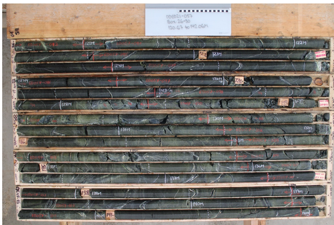
Figure 4: DDED21-057: Serpentinized peridotite, dunite host unit with trace disseminated sulphides
