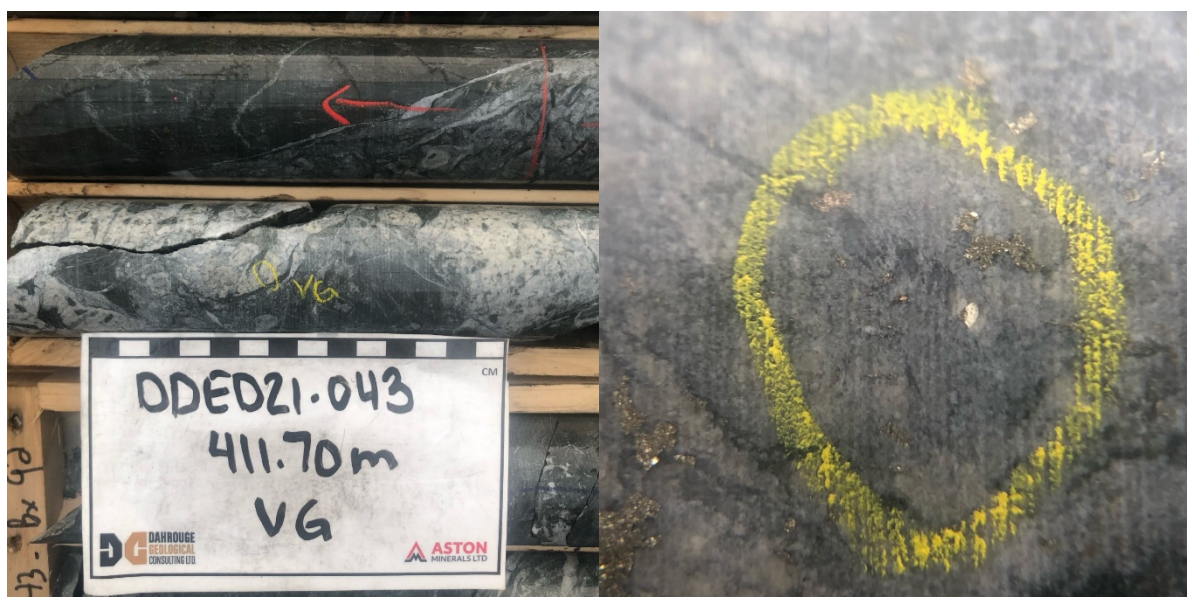
Figure 9: Logged visible gold within quartz-carbonate veining associated with arsenopyrite
