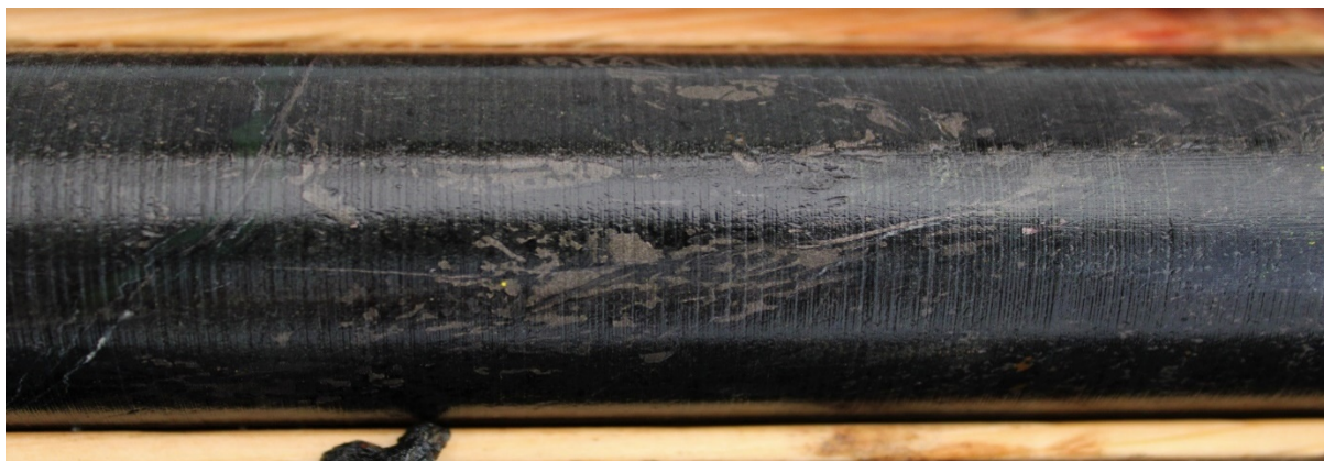
Figure 17: DDED21-059: blebby (pyrrhotite-pentlandite) 5% within fine grained peridotite at 86m
