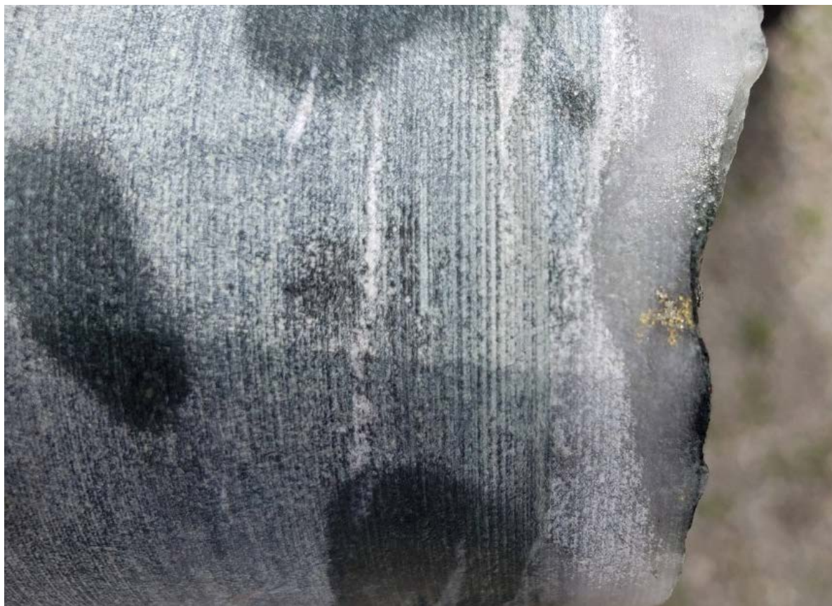
Figure 6: DDED21-035 - visible gold intersected from 101.78m at Edleston Main
