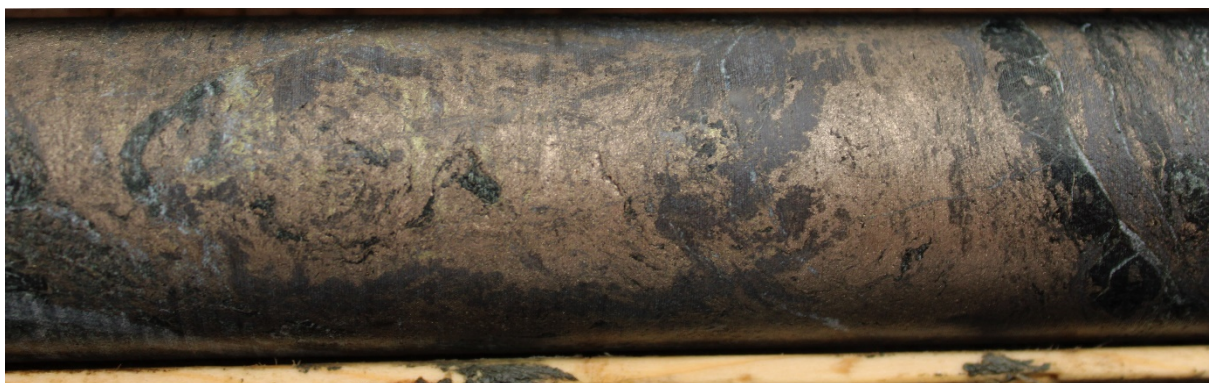
Figure 16: DDED21-059: semi-massive (pyrrhotite-pentlandite-chalcopyrite) within fine grained sheared peridotite at contact with rhyolitic tuff at 54.5m (dry core)
