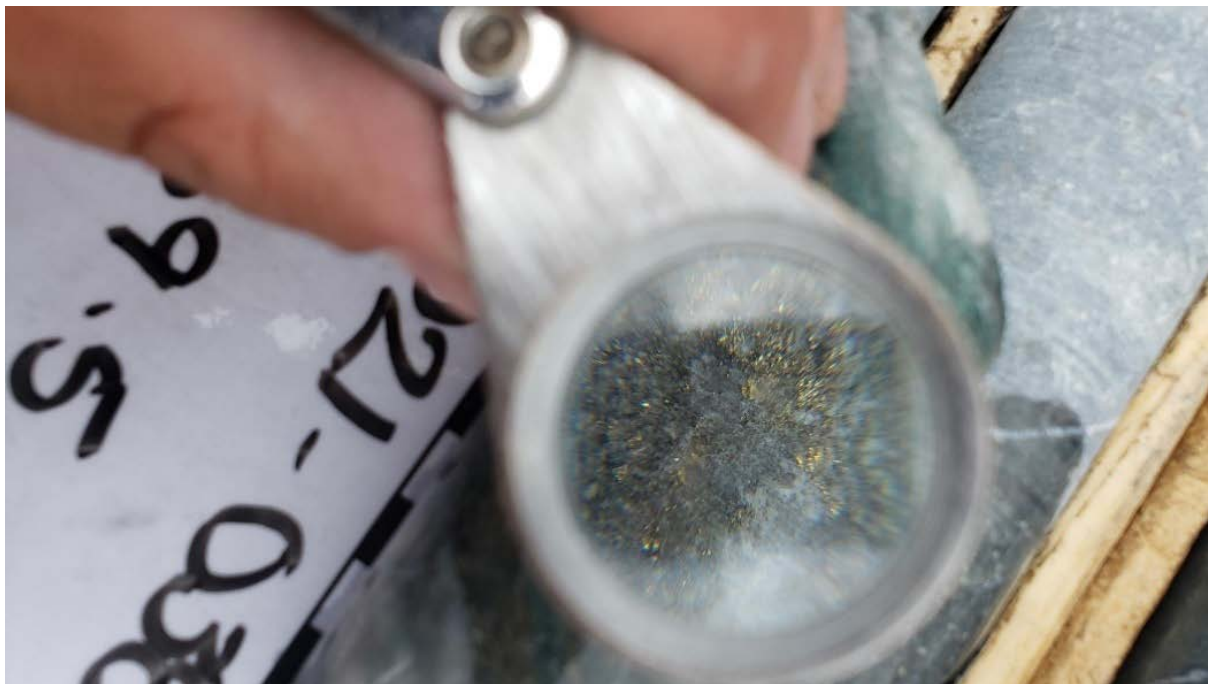
Figure 5: DDED21-038- Visible Gold Intersected from 469.5m at Sirola Prospect
