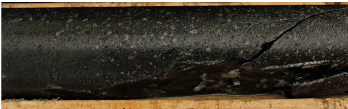
Figure 18: DDED21-059: Coarsely disseminated sulphide (pyrrhotite-pentlandite) 5% within medium grained peridotite from 180.5m
