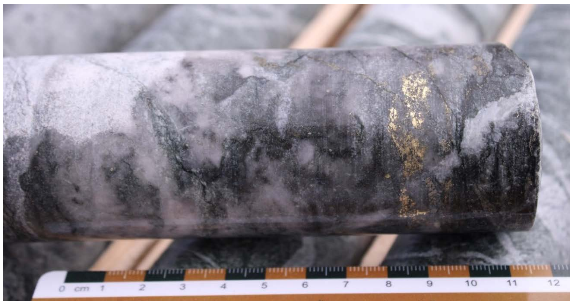
Figure 3: Interval of coarse visible gold veinlets at 362m (DDED21-003)
