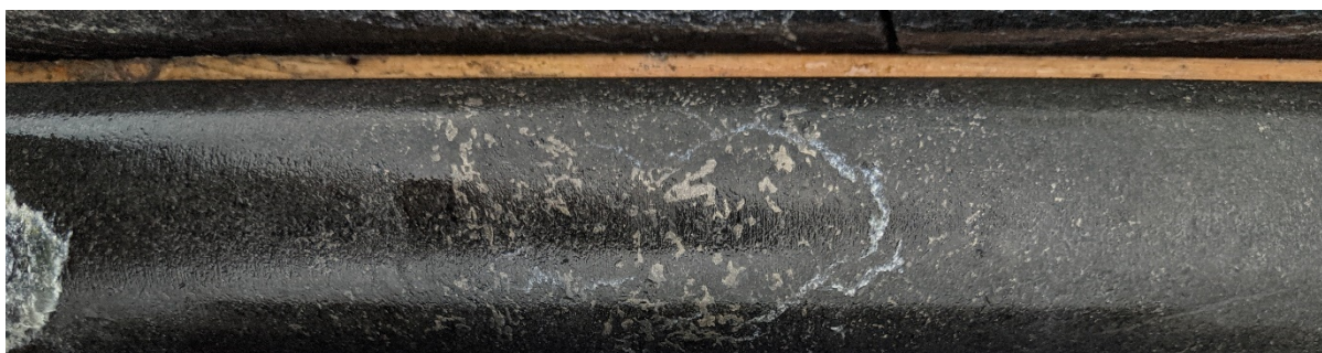
Figure 20: DDED21-059: Fine disseminated to medium grained blebby (pyrrhotite-pentlandite) 5% within peridotite from 256m
