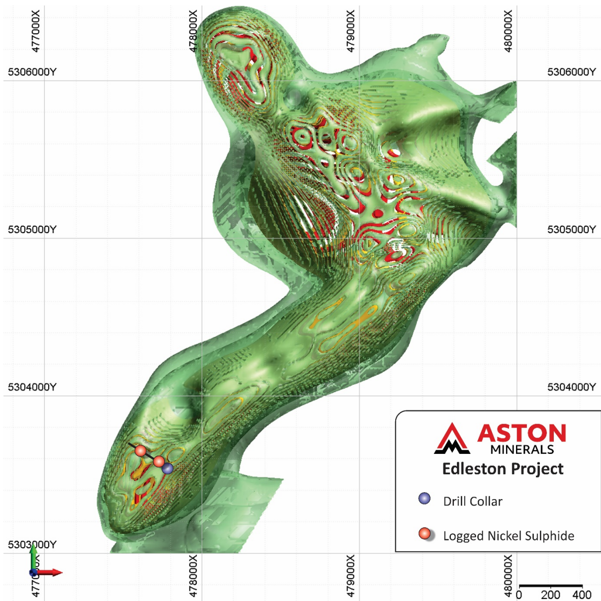
Figure 15: Magnetic Inversion Model- Plan View of Boomerang Target & Recent Drilling
