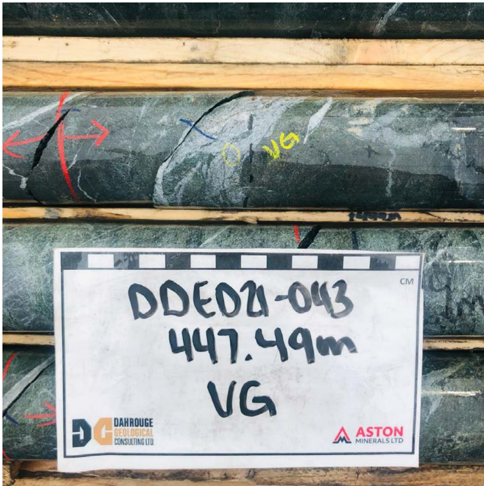
Figure 10: Logged visible gold within carbonate vein associated with pyrite
