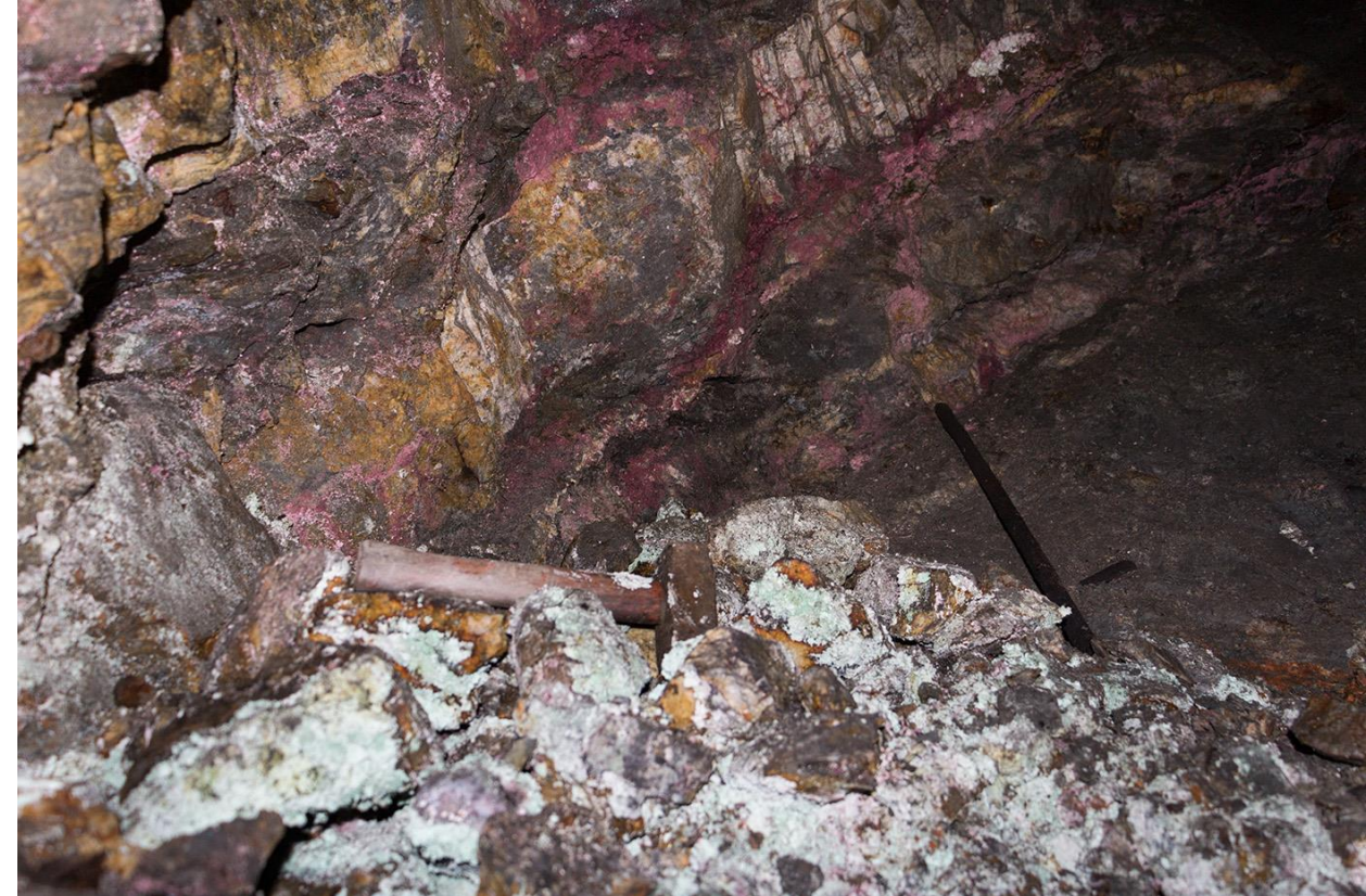
Joremeny Adit- Erythrite Coating on Co-Ni Mineralised Structure, Massive Sulphide Mineralisation in Mullock- J3 Rise East Joremeny
