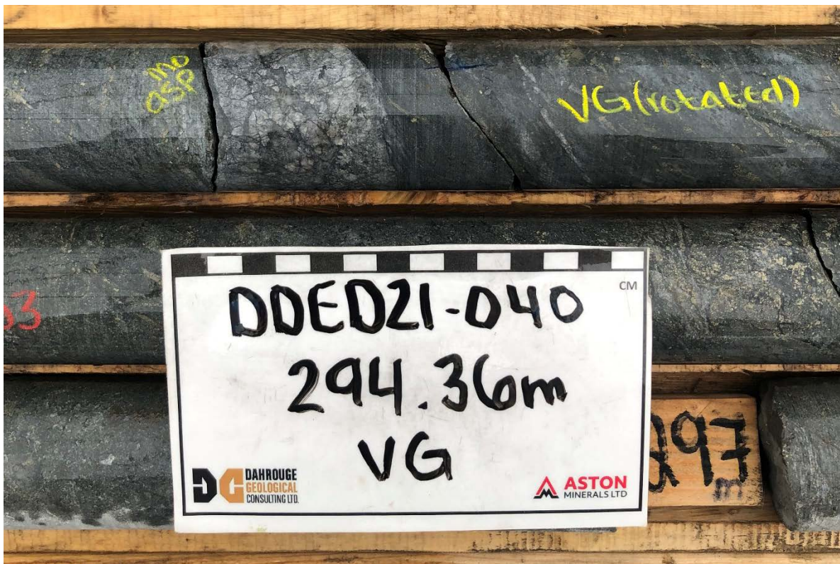
Figure 6: Visible gold within quartz-carbonate vein associated with arsenopyrite and molybdenum
