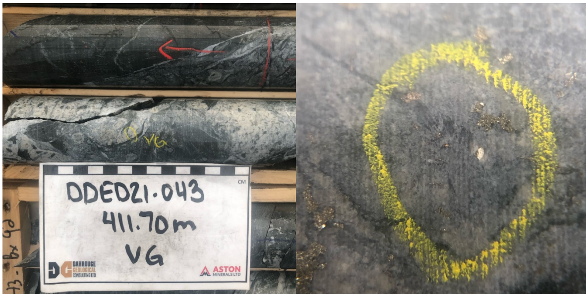
Figure 3: Logged visible gold within quartz-carbonate veining associated with arsenopyrite
